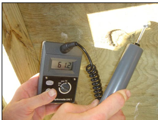
Figure 3b. A non-intrusive/non-penetrating moisture meter—recommended for initial and interim moisture readings.
